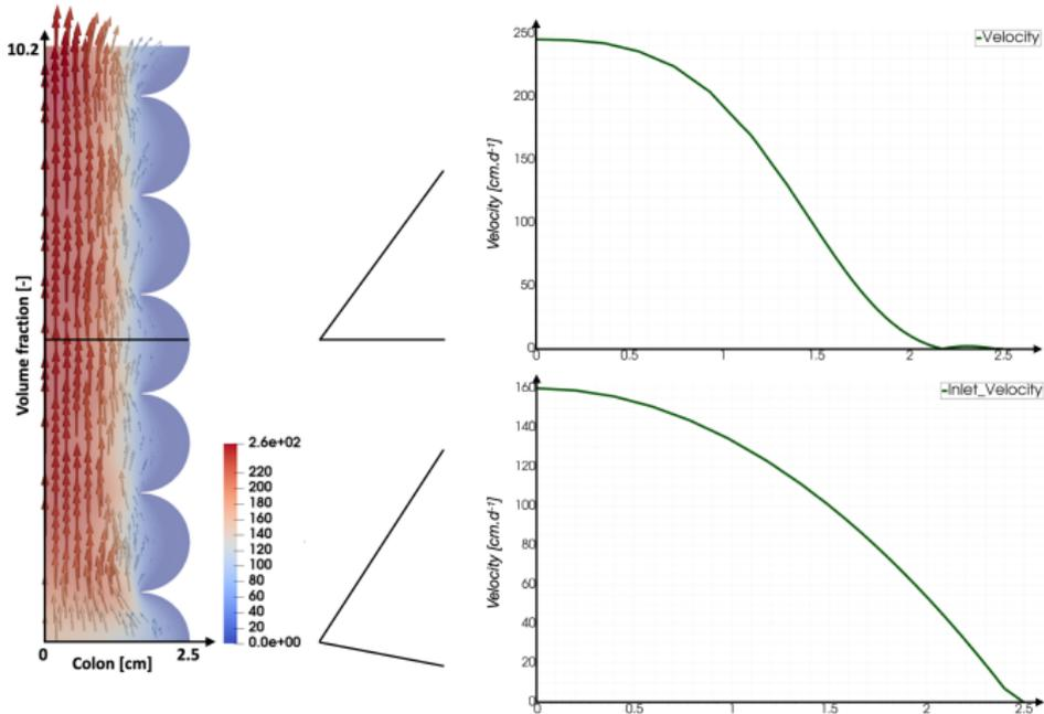
*Velocity with vector field representing flow direction and radial sections.*
